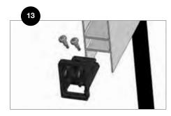
Position the top brackets into the H-bar, making sure they are inserted completely.
