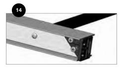
Secure using the supplied #10 x 5/8-in. selfdrilling screws.
