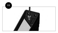
Using integrated screw template, secure with the supplied #10 x 5/8-in. self-drilling screws.
