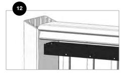
Position the top rail over the infill assembly, and carefully lower into place.
