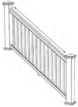
Building codes are very specific on allowable angles and widths. It is very important to consult with your local building code officials and plan your stair layout accordingly. Leave adequate space for graspable hand rail if applicable.
