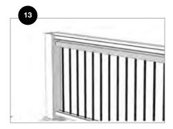
Position the top rail over the H-bar, and carefully lower until fully seated.
