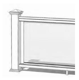
Note: Prepare top rail, bottom rail and H-bar and attach bottom rail brackets to the posts following standard 6-ft. line railing installation instructions prior to CVS installation.
