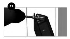
Assemble and attach the crush block following standard line railing instructions.
