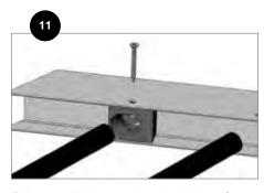
Fully seat all balusters into the holders. Secure an end baluster first using the supplied #8  $\times$  1-1/2-in. flat head self-drilling screws.
