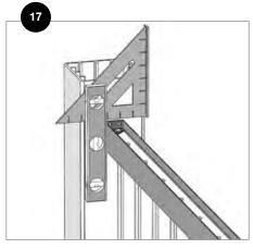
Center the H-bar on the post and check rail for plumb.
