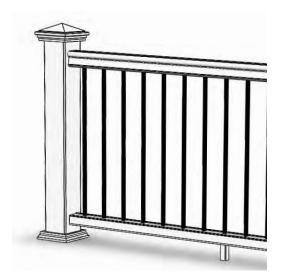
Note: Prepare top rail, bottom rail and H-bar and attach bottom rail brackets to the posts following standard 6-ft. line railing installation instructions prior to aluminum baluster installation.
