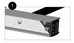
Secure with self-drilling #10 x 5/8-in. screws. Do not over tighten.
