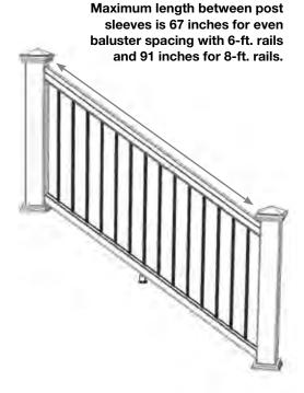
Install 4x4 posts in the pre-determined locations, cover with post sleeve and verify spacing. Posts should be plumb in both directions. Place post sleeve base moulding over post sleeve and slide it down to the deck surface.
