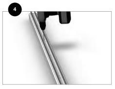
Predrill the remaining holes and secure with a #10 flathead screw.
