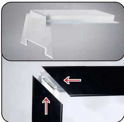
Step 1: Miter Top Rail Miter top rails to create a 90 degree corner and slide splice into each end of the rail.
