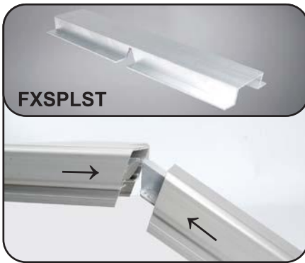
Series 200 - Stair Splice Splice slides into each end of the rail. Bend splice to the correct angle of the stairs and secure splice into place with 8 ea. screws.
