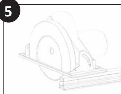
Cut top rail to length measured in step 4. When cutting a stair top rail ensure the angle of the stair is set on the saw.
