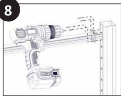
Drive a provided screw through each hole in the rail mounting bracket into the post.
