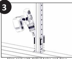
Align post with drilled holes and drive mounting bolts into place.
