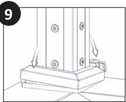
Place a trim ring around the bottom of each post rotating the halves into a position where they engage one another.
