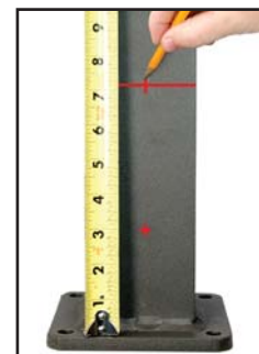
Mark all remaining holes 4-5/32" on center from each other
