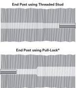
2. Slide the stainless steel washer onto the threaded stud (smaller for metal post, larger for wood) and start the brass locknut onto the threads as far as possible by hand. Feed the cable through the end post, pulling the threaded stud into place.
