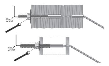
2. Tension all cables to desired amount in sequence, beginning with the center cables, moving up and down toward the top and bottom.
