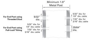
Intermediate posts are drilled on the angle.
